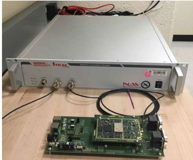
Figure 2: IFEN multi-GNSS signal simulator (top) pictured along with a Septentrio AsteRx4 receiver OEM development board (bottom).
