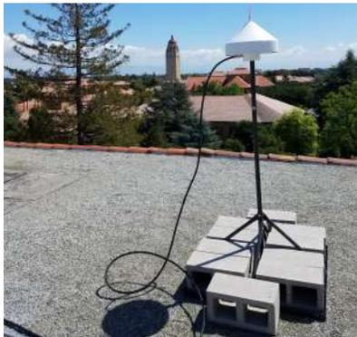
Figure 5: Septentrio Choke Ring antenna mounted at Stanford University
