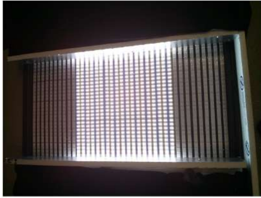
Figure 10: Light-box after a 15 minute operation. The two band of LED strips on the peripheries were automatically switched off by the LED controller.
