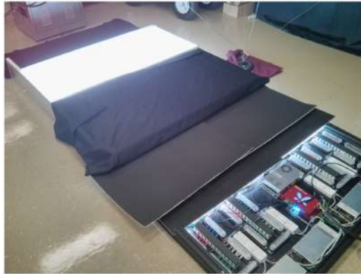
Figure 9: Light-box with all RGB and white LED strips at maximum voltage setting. Sections of light-box not being tested were covered with black cloth.
