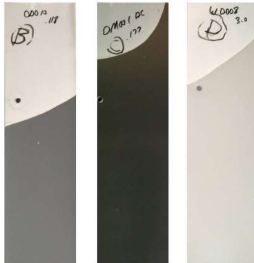
Figure 2: Segments of the three diffuser plates used in the experiment; the plate with manufacture marking of (00010, 0.118) is referred to as Plate B, (0M001DC, 0.177) as Plate C, and (W0008, 3.0) as Plate D.
