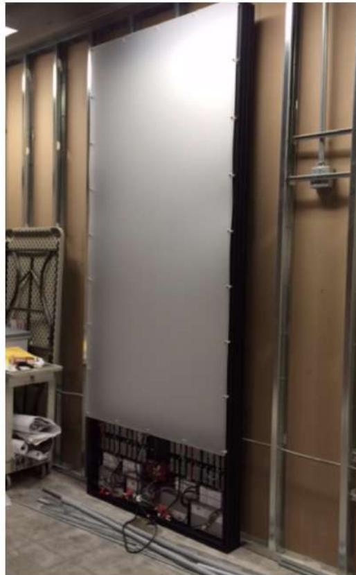
Figure 6: Full-scale prototype light-box device mounted vertically to a wall at the Space Rendezvous Laboratory.
