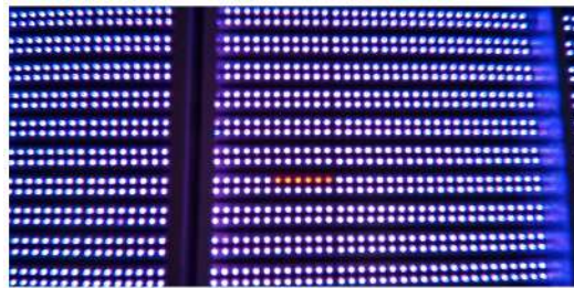
Figure 11: Malfunctioning RGB LED strips in the light-box, this particular section was not used in the Radiance Output Test.
