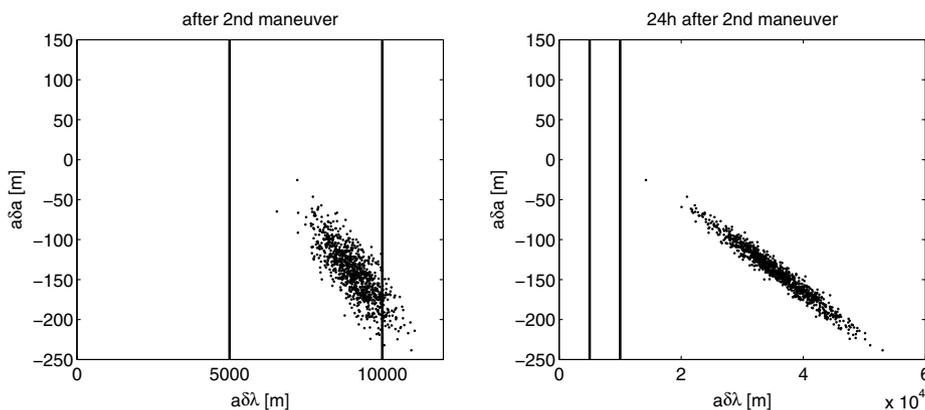
Fig. 4 Residual  $a\delta a$  in dependence of mean tangential separation ( $p = 0.0732231$  m/s, no differential drag).
