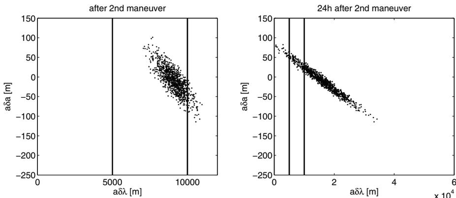
Fig. 5 Residual  $a\delta a$  in dependence of mean tangential separation ( $p = 0$  m/s, drag included).
