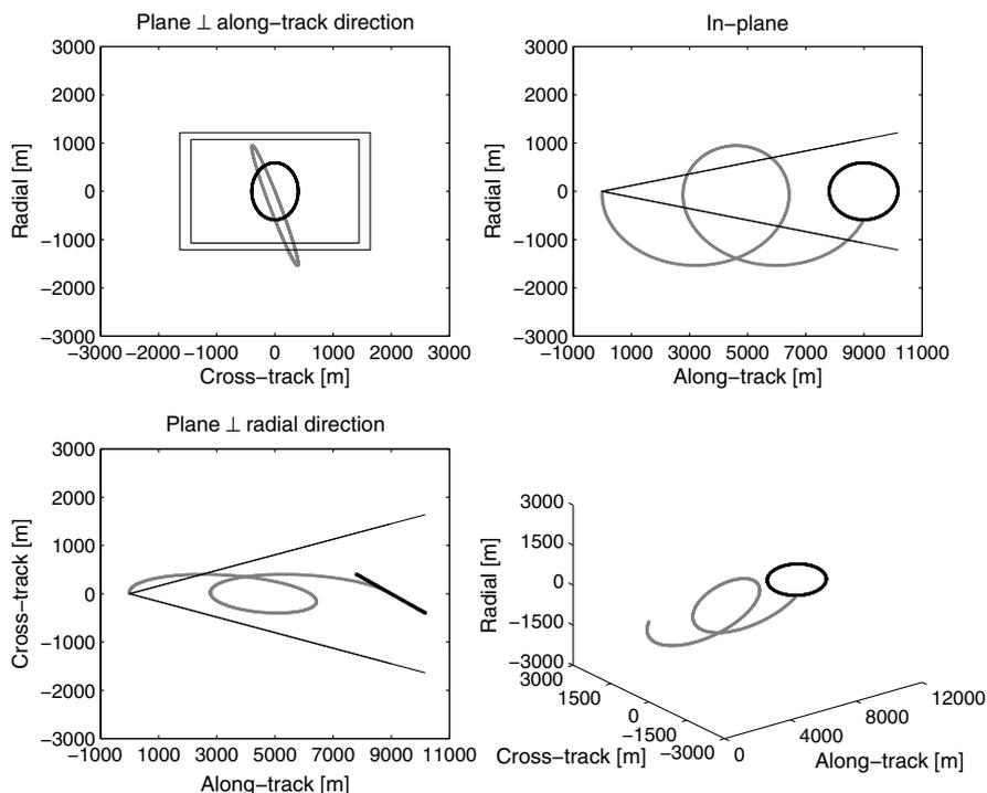
Fig. 3 Example of the feasible baseline of Eq. (16) with delta-v of Eq. (17).
