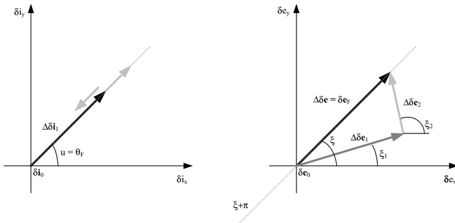
Fig. 2 Sketch in the ROE space of the maneuvering scheme of Eq. (7) to achieve passive safety.
