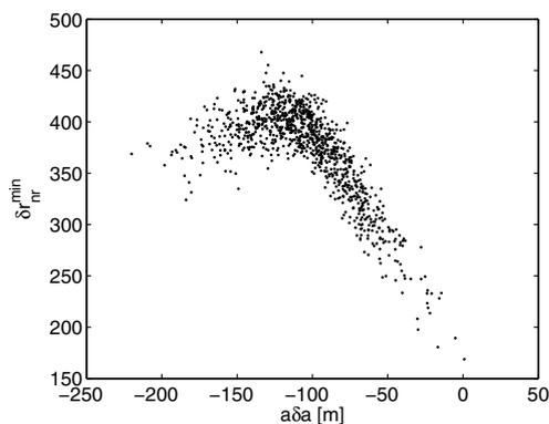
Fig. 8 Minimum cross-track distance as a function of the final  $a\delta a$ .
