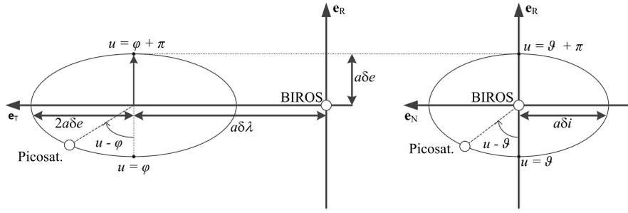
Fig. 1 Sketch of ROEs and their relation to the relative motion in the RTN frame.
