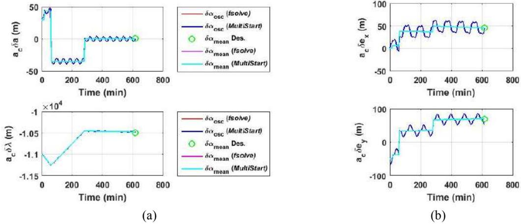
Figure 7. Full maneuver: (a) relative mean semi-major axis and longitude; (b) semi x- and y-component of mean relative eccentricity vector.
