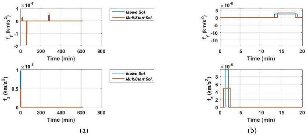
Figure 9. Control profile for out-of-plane maneuver (a) and zoomed-in view (b).
