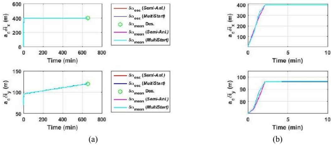
**Figure 5. Out-of-plane maneuver: x- and y-components of the mean relative inclination vector (a) and zoomed-in view (b).**
