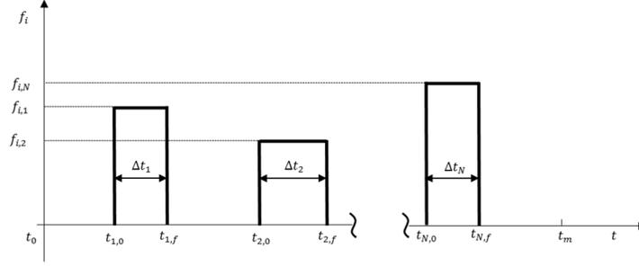
**Figure 1. Continuous on/off control profile.**
