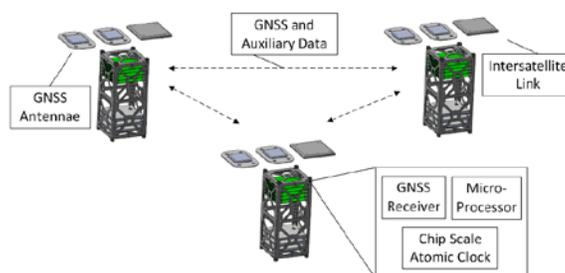
*DiGiTaL consists of a plug-in ready multi-GNSS hardware/software 0.5U unit capable of integration with most satellites enabling peer-to-peer decentralized navigation accuracy at the centimeter-level over separations up to hundreds of kilometers.*
