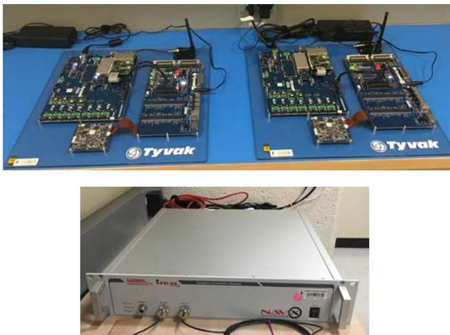
DiGiTaL is validated on two Tyvak flatsat development boards (top), each consisting of a Novatel OEM628 Multi-GNSS receiver, an Endeavour flight computer (800 MHz), and a UHF intersatellite radio. GNSS signals are generated using an IFEN GNSS Signal Simulator (bottom), allowing for GPS L1 and L2, Galileo E1, and BeiDou B1.
