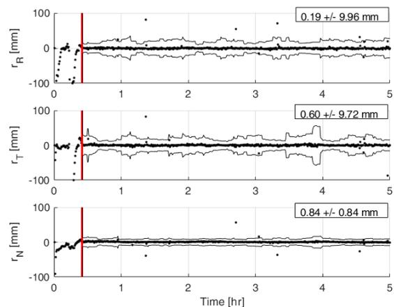
DiGiTaL's relative position navigation errors and 3 $\sigma$  covariance bounds for two spacecraft in the frame aligned with (R)adial, (T)angential, and (N)ormal directions. Results show sub-centimeter level accuracy obtained in real-time on-board CubeSat avionics. Red line indicates initialization of carrier-phase integer ambiguity resolution.
